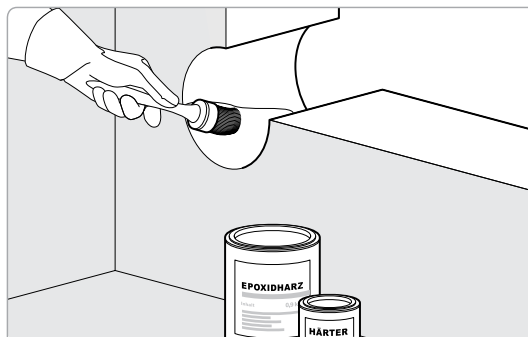
Figure 9: Protect the Bore Wall with Epoxy Resin
